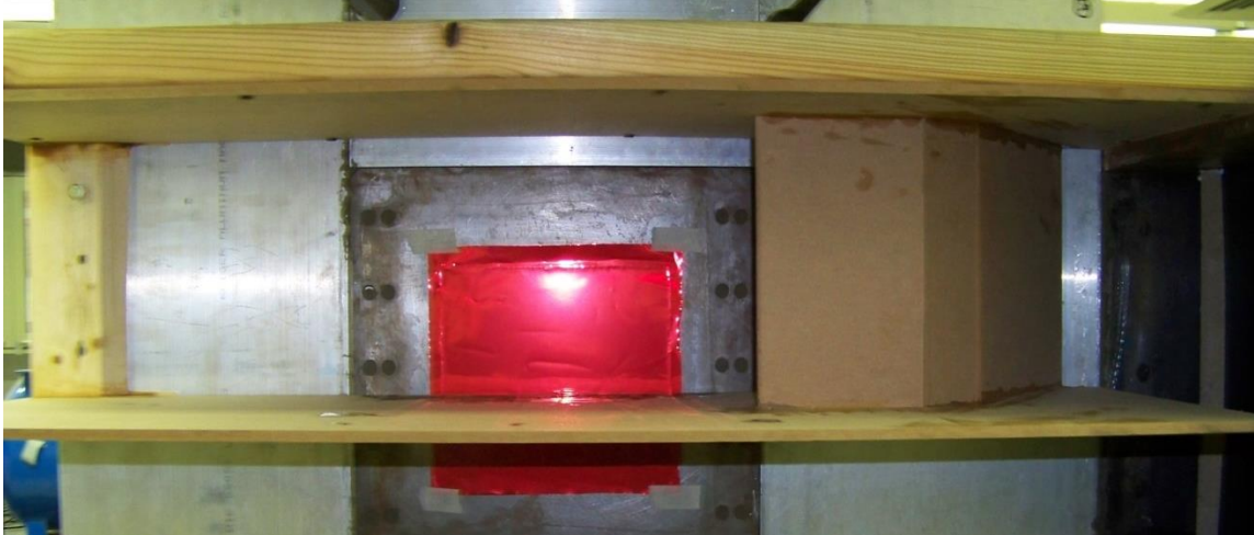
Figure 3.10. Picture of vertical splitter in place.
